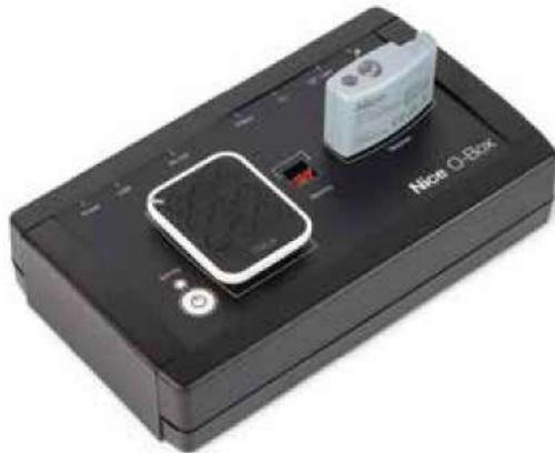
**O-Box is the multi-function interface which, thanks to the dedicated software “O-Box Software Suite”, enables the configuration and programming directly from the PC or PDA, practically and intuitively, all transmitters, receivers and other Nice control devices.**
